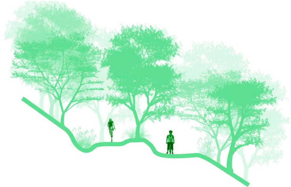
Figure 4.2.17: Example of mountain bike trail switchback (left); cross-section of switchback (right). (Source: Appalachian Trail Conservancy, n.d.)
